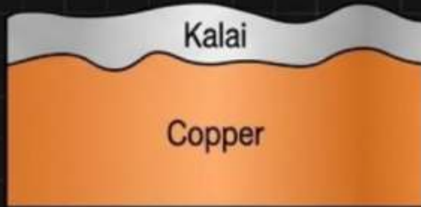
Tin-lined Cu/Brass (Outer metal + inner Kalai layer)
